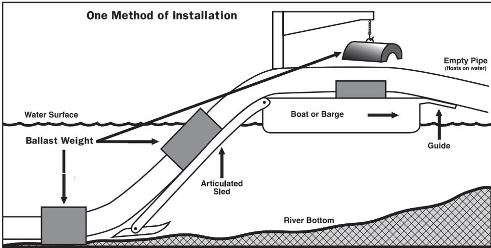
**Figure 1** Submerging a heavily weighted pipe from a barge
