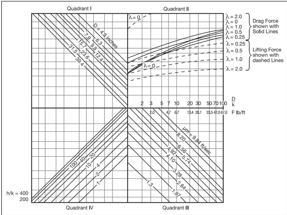
**Figure A-2-2** Graph for the estimation of drag and lifting forces on underwater pipes when the flow rate of the current times the pipe diameter is 2.7 ft<sup>2</sup>/sec, or greater
