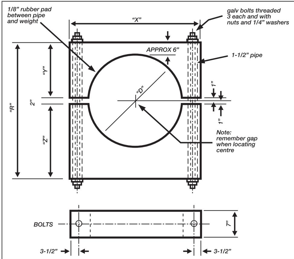
**Figure A-3-2** Typical Detail of Concrete Ballast Showing 1-inch Gap Between Ballast Sections
