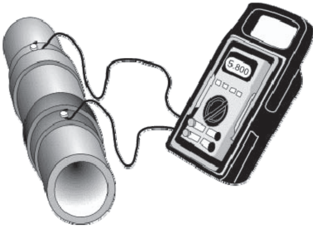
Figure 6 Typical Electrofusion Control Box and Leads with Clamps and Fittings
